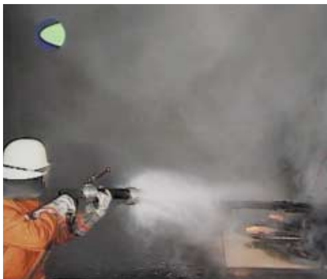
A Fogtec high pressure water fogging gun in action on a test fire.
